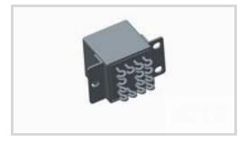
Type of Control: Fixed Time Delay Relay Input Voltage: 28 VDC Time Delay Relay Contact Current Rating: 10A@28VDC A, 115VAC A Mode of Operation: Delay on Operate Delay Time: 1 second
